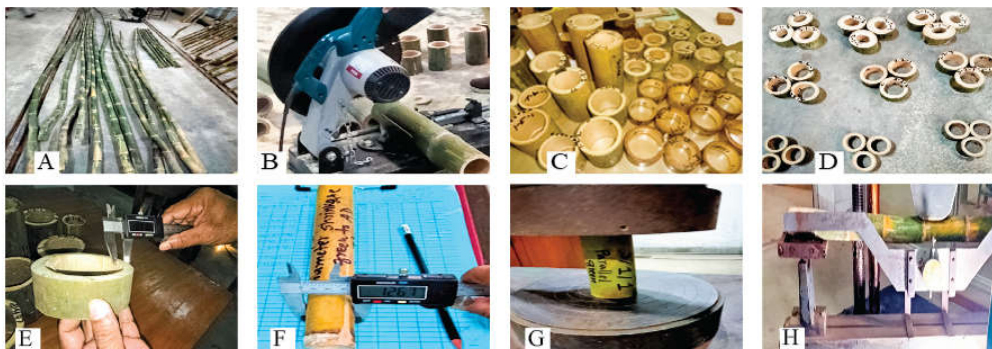
Figure 1. Different steps of The determination for physical and mechanical properties of Thai bansh (A-H).
