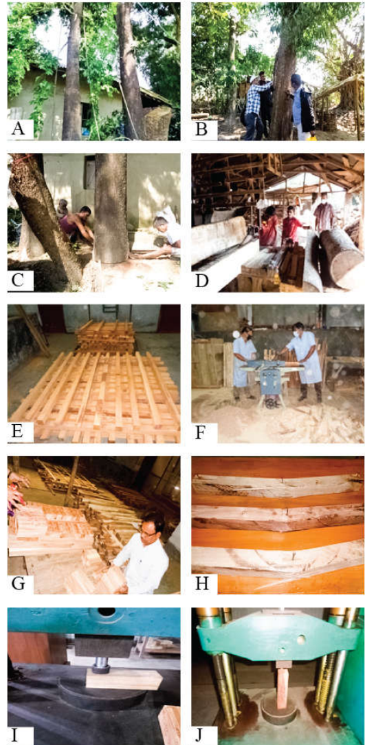
Figure 1. Different steps of the determination for physical and mechanical properties of Mahogany and Acacia hybrid wood.
