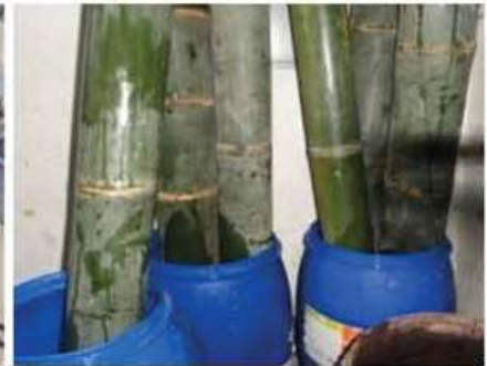
Bamboo preservation technique by Sap-displacement method
